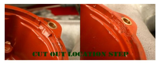
To locate the distributor cap rotationally, moulding features in both the Bosch and aftermarket (see images above) can be lined up with the notch originally intended for the location step:
