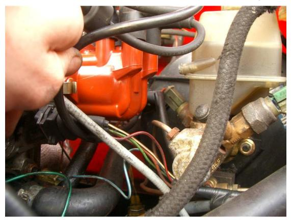
Tthe standard leads can be used without modification and the adjustments required to the ABF cap are minimal. It is quick converting it straight back to the straight exit cap if required.
