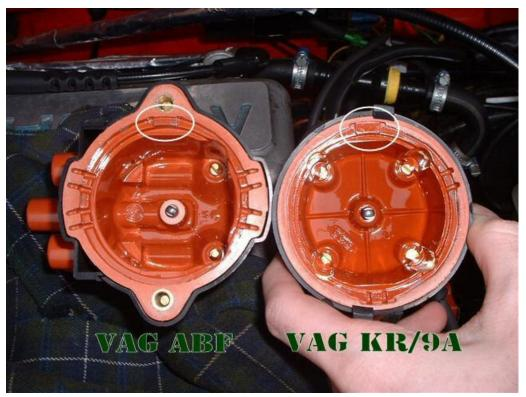
Main differences between the Bosch (VAG) caps being outer black shrouding, but also the Bosch ABF cap has a different internal contact design. Either way it doesn't matter, both Bosch and aftermarket ABF caps (in this case GS&F) can be used no problems.
